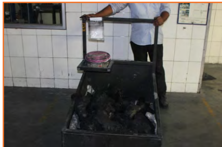
Move compound to next operation or storage area after quality inspection
