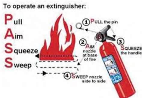
Fig. 8.4.10. Method of operating Fire extinguisher
