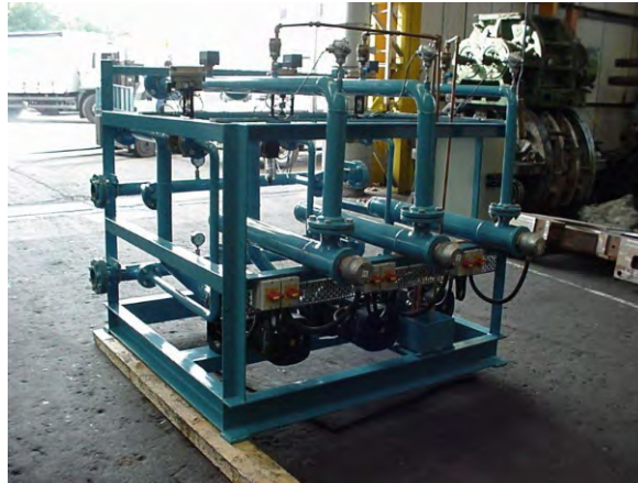
Fig. 1.5.5. Temperature Control Unit
