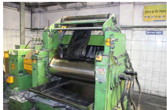
Fig. 4.1.1 Curing agent mixing in mixing mill
