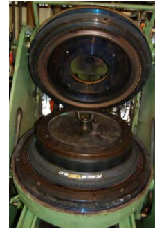
Fig. 2.2.1. Mould loading in tyre moulding machine
