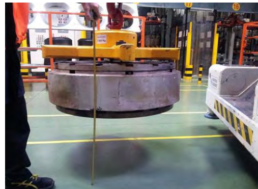
Fig. 2.2.4. Carrying mould with the help of Crane
