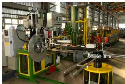
Fig. 1.5.2. Tyre bead winding process
