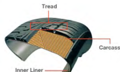
Fig. 1.4.4. Bias tyre internal construction
