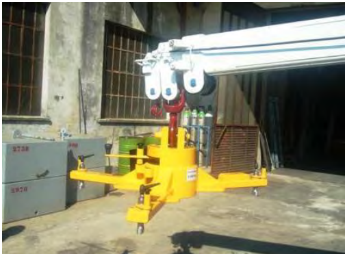
Fig. 2.2.3. Crane arrangement for mould carrying clamp
