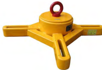
Fig. 2.2.2. Clamp for tyre mould movement
