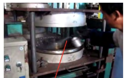
Fig. 2.2.8. Spraying mould release agent
